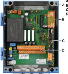
A AMI TransmitterB Slot for interfacesC Frontend PCBD Screw terminals
